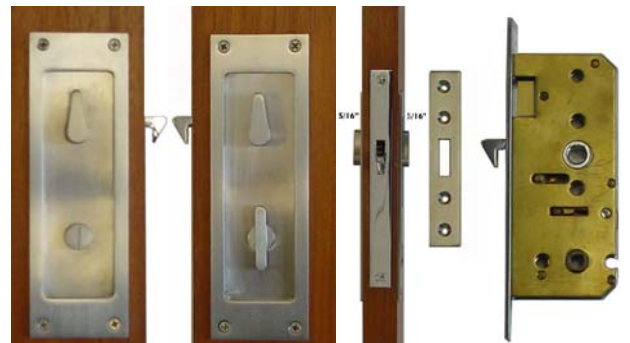
Flush lever set #13.CSB custom made with lock #16.401 and strike #14.48S MINIMUM DOOR THICKNESS: 1 1/8" Lever extend 5/16" from surface on each side of door
