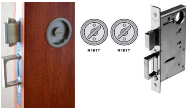
SET: 13.PAR161 Passage set with full mortise mechanism with spring loaded edge pull ; ROUND flush pull with thumb-turns; 2 3/8 inch diameter. MINIMUM DOOR THICKNESS: 1 3/8"
