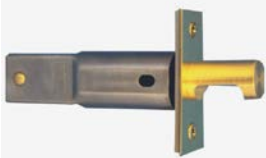
13.161PDP Edge pull Mechanism for pocket doors thickness casing: 1 inch. For 1 3/4" thick doors. Pull 5/8" diameter; spring loaded.
