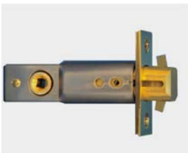
13.161PDL Hook bolt for pocket doors; specify 2 3/4" or 2 3/8" backset; Thickness lock casing: 1 inch; for 1 3/4" thick doors
