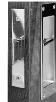
SET: I3.PR001 Privacy Pocket Door Lock with thumb-turn on inside and indicator outside; MINIMUM DOOR THICKNESS: 1 3/8"; Backset 2 1/2"
