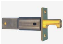
13.161PDP Edge pull for pocket doors thickness casing: 1 inch. For 1 3/4" thick doors. Pull 5/8" diameter; spring loaded.
