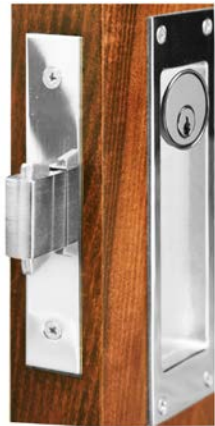
SET: I3.EP001 Entry Pocket Door Lock with Key outside and flush lever inside; MINIMUM DOOR THICKNESS: 1 3/4"; Backset 2 1/2"
